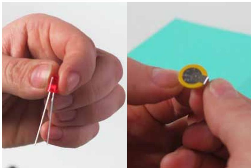
2.1 Its always a good idea to check your components before you paint them into the circuit. So put positive leg of the LED to the positive leg of the battery and the same with the negative legs and your LED will light up. If it doesn't double check you have everything the right way round.
