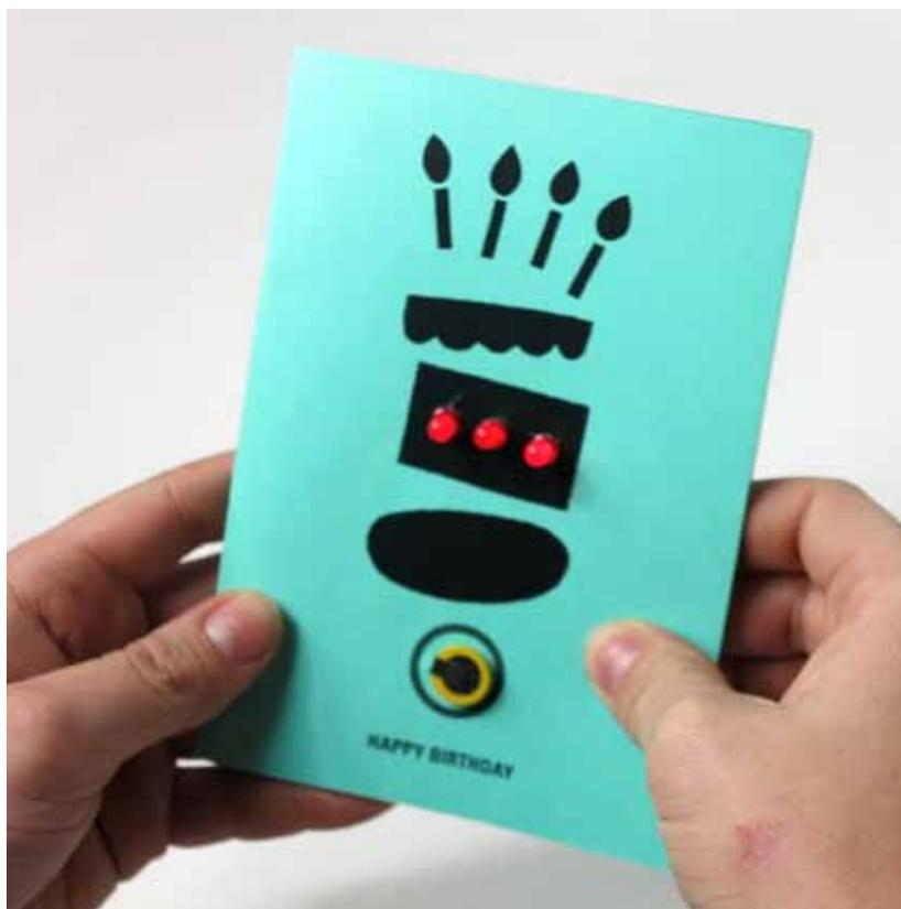
5.2 Now fold your switch in half and add glue to the half without the bare paint on and stick to the card body to create your finished switch.
