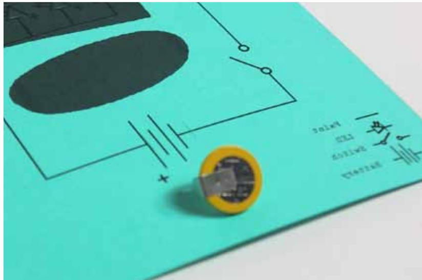
2.2 Line up the battery with the diagram to make sure you have it the right way round.
