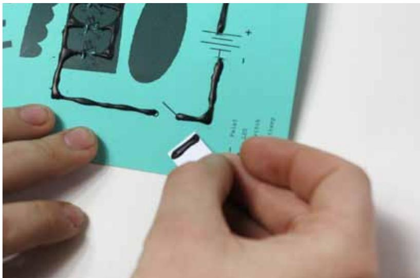
5.1 Then hold the switch in place and turn over and check that the LEDs are on.
