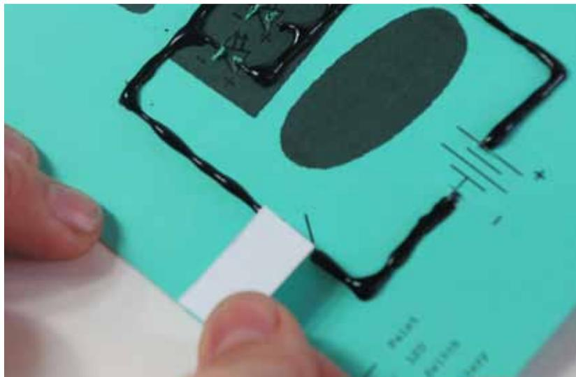
4.1 Next we're going to paint it with a patch of Bare Paint so that when it closes, it makes a bridge across the gap and turns the circuit on!
